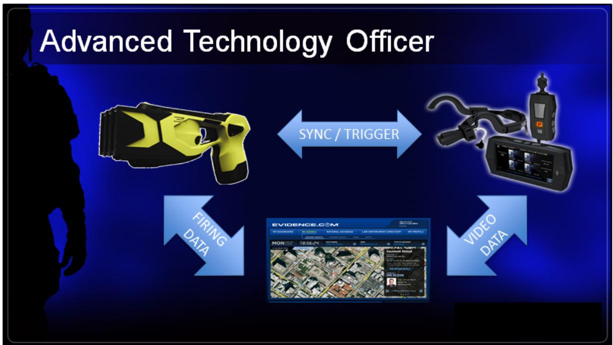
In the illustrated TACOM system, the data from the CEW and on-officer camera could be communicated to a computer-based evidence system (TASER's Evidence.com system, as shown). This coordination allowed for synchronization of data recordings from connected devices when transferred to Evidence.com.
